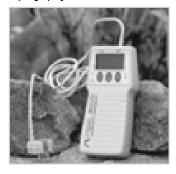
These devices measure the concentration of exhaled CO2 from the lungs. The mere presence of CO2 indicates proper tracheal tube placement. The lack of CO2 detected may mean that the tube is in the esophagus, especially if the patient's lungs are receiving a good blood supply.
